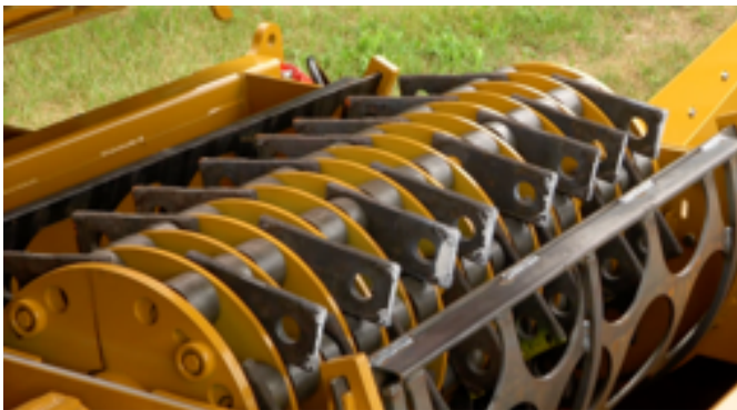
The mill and the rotor. The screen behind them is what turns “chopped” into “chopped to a number.”
