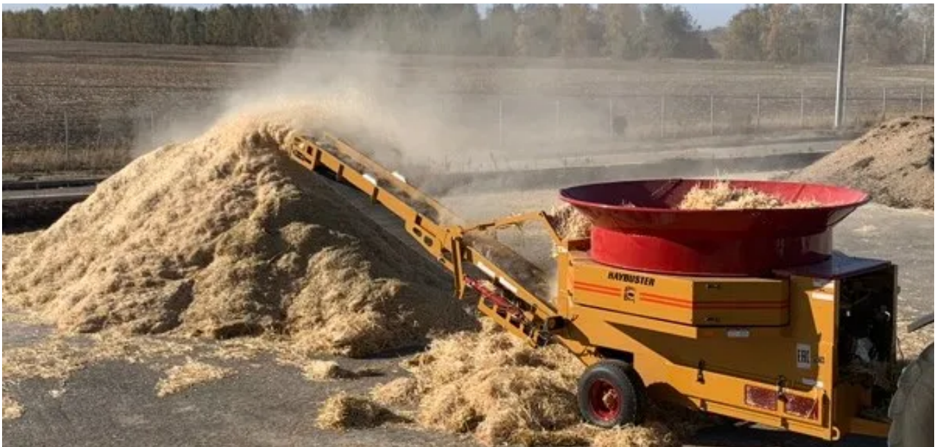
A HayBuster tub grinder at work. The same machine named in the study's methods section.
